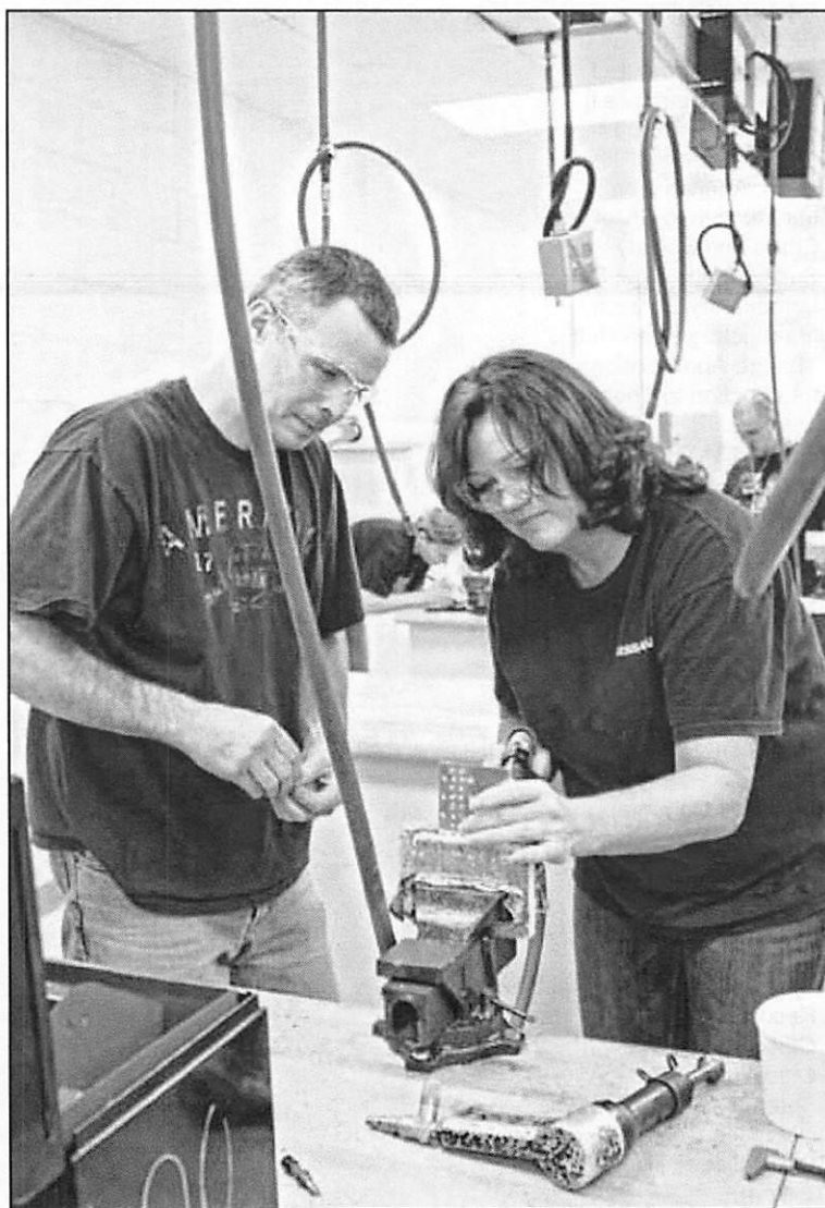
Two AAC students work on a sheet metal structural project, known as a flush patch, by riveting the sheet metal together.
